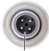
Alignment pin in the Wellhead and logger connectors
